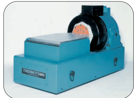
Above: A DS-2250 slip table configured for horizontal vibration.
